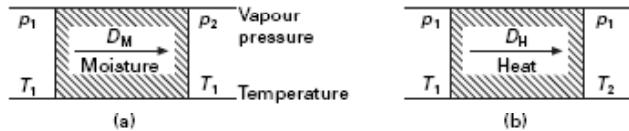
9.12 Steady-state conditions: (a) vapour pressure gradient at constant temperature; (b) temperature gradient at constant vapour pressure.
